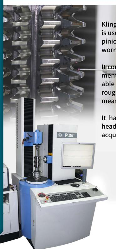
Klingelnberg P26 Measuring Machine is used to inspect the cylindrical gears, pinion type cutters, shaving cutters, worm wheel hobs, bevel gears etc.
